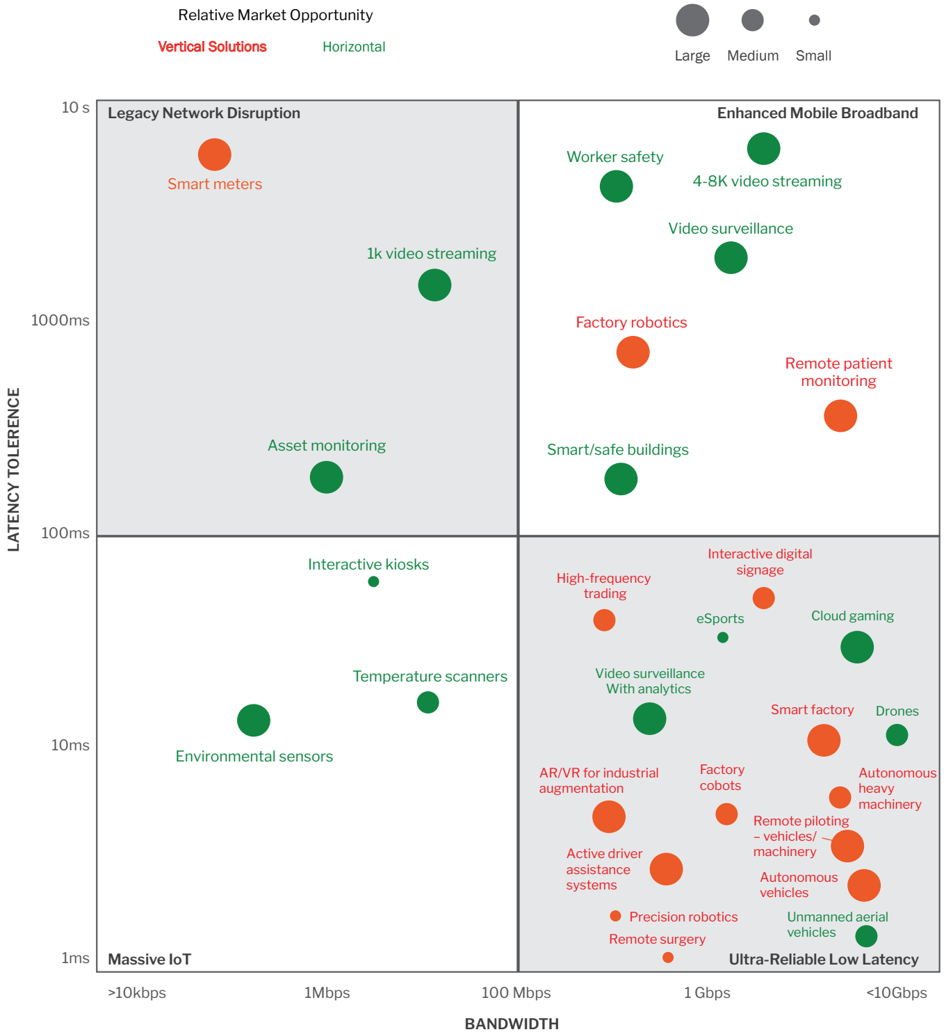
Figure 4: Plotting horizontal and vertical 5G edge cloud network use cases
